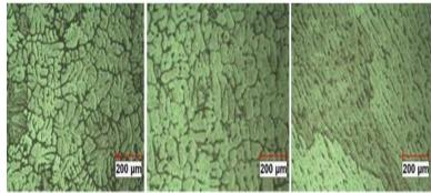
(a) (b) (c) **Fig. 2** Optical micrographs at 100X magnification of fabricates composites (a) Al-10% TiO2-0.5% GO (b)Al-10% TiO2-0.75% GO (c) Al-10% TiO2-1.0 % GO
