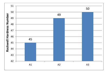
**Fig.3** Rockwell hardness test results where A1: Al-10%TiO2-0.5%GO, A2: Al-10%TiO2-0.75%GO, A3: Al-10%TiO2-1.0 %GO
