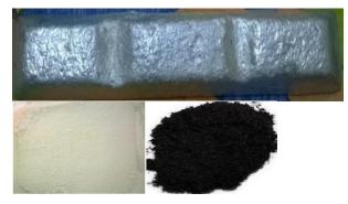
**Fig.1** Aluminum 7075 alloy ingot, TiO2 powder and Graphene Oxide powder
