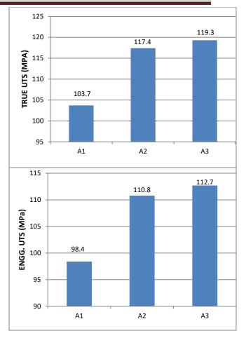
Fig.4 Variations of True stress and Engineering stress with composite specimens
